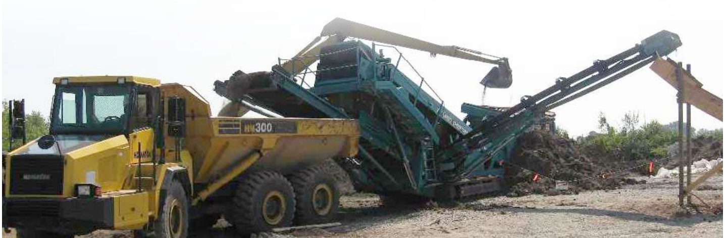
Soil sifting operation conducted by MKM to separate munitions debris and other metals from soil.
